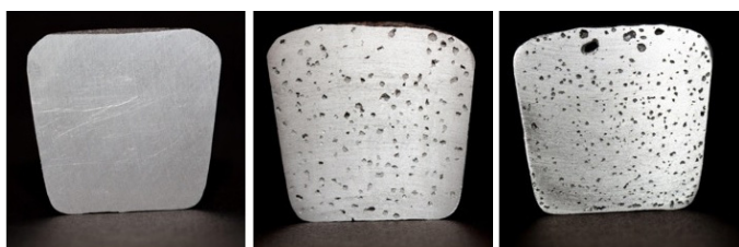
Fig. 4. Sample solidified in partial vacuum: Directly casted sample (left), 2× remelted (middle), 4× remelted (right)
